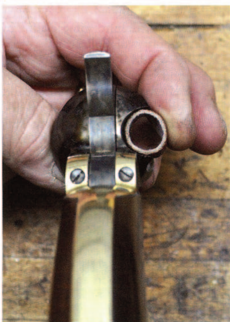
GRINDING THE EJECTION CHANNEL.
